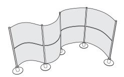
The panel curvature is determined by moving the uprights closer or farther apart.
