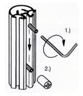
1 Insert threaded stud into center grooved channel (see figure above) AFTER ascertaining desired shelf position, screw threaded stud in so that it seats all the way to the back of the grooved channel.
